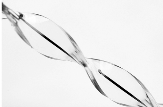
By encasing gallium alloys in flexible plastic, researchers have created a deformable and tunable antenna. Image credit: Michael Dickey (North Carolina State University, Raleigh, NC).
